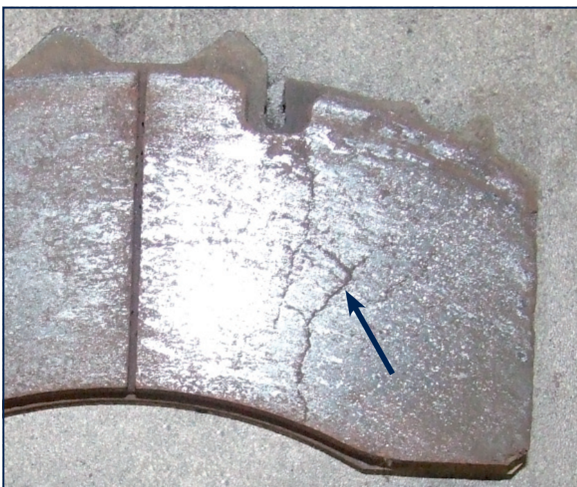
Figure 4: Cracks in the permissible area of the lining surface
