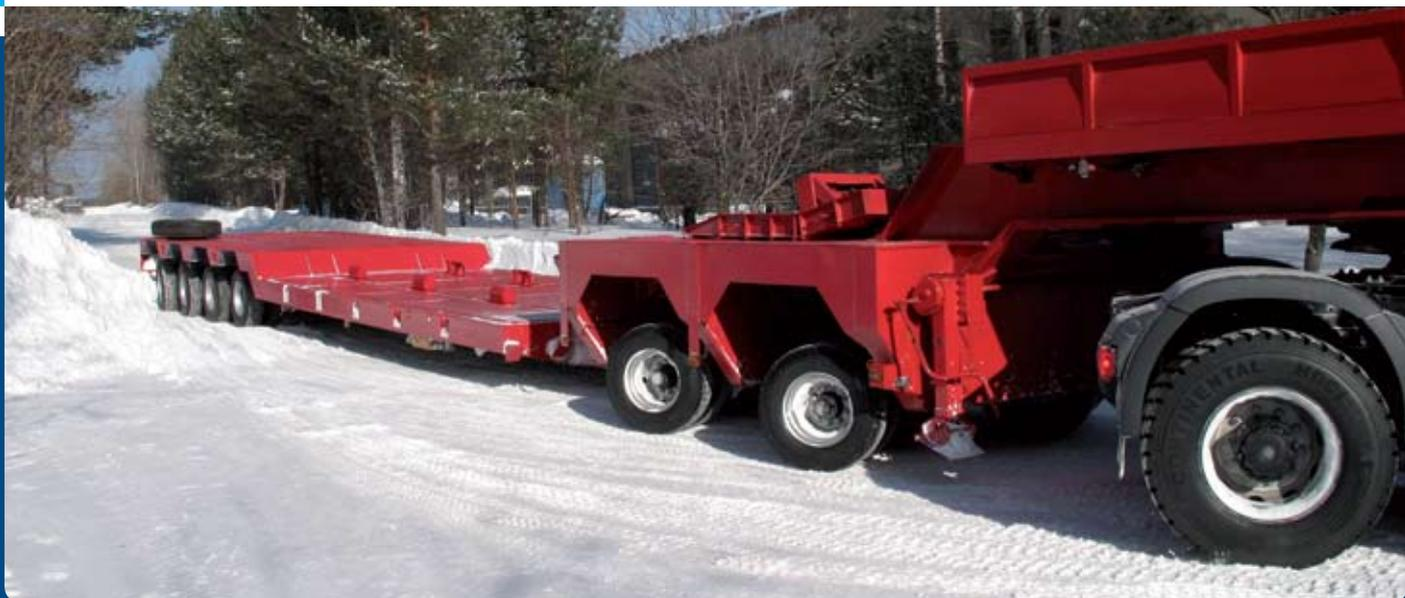
***The oscillating axle suspension for extremely heavy transport
