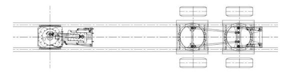
The TRIDEC HS steering system is a hydraulic steering which is suitable, for example, for transporting construction materials or ballast and other trailers used in heavy industry. The HS system can also be used for extendible trailers and self tracking dollies.
