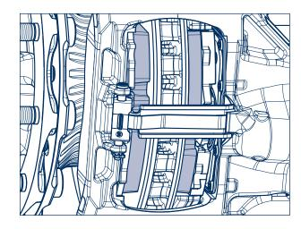
The brake lining thickness can be checked by the position of the brake caliper in relation to the welded-on brake anchor with the wheels mounted (approximate wear indicator).
