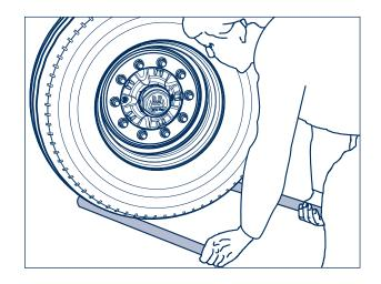
If a play of the bearing is detected on the **ECO Plus 3 Unit:**
