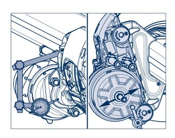
Press the brake caliper <u>upwards</u> and determine the play of the bearing on the dial gauge.
